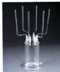
6-Way Distribution Activated Carbon Tank
