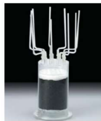
9-Way Distribution Activated Carbon Tank (This photo shows activated carbon filled.)
